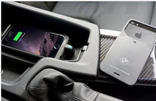
Source: Aircharge; Automobiles such as BMW offer in-vehicle Qi wireless charging and branded products
